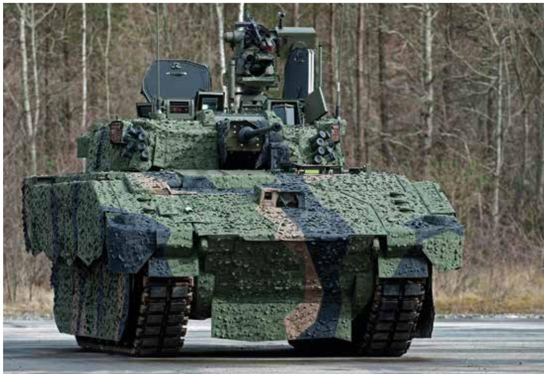
*Pictured is the new AJAX prototype shown near its future assembly site in Merthyr Tydfil, Wales. Each AJAX platform variant has extensive capabilities, including acoustic detectors, a laser warning system, a local situational awareness system, an electronic countermeasure system, a route marking system, an advanced electronic architecture and a high performance power pack. Photo: Richard Watt, Crown Copyright*
